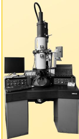
120kV TEM capable of resolving down to 0.3 nm; the system is heavily used in nano-scale investigations of interfaces and thin films. An Oxford EDX attachment is added allowing high spatial resolution elemental analysis.
