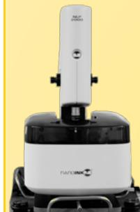
Nanolithography instrument capable of depositing a wide variety of materials with sub-micron accuracy and precision. Used for multiplexed protein printing, biosensor functionalization, nanopatterning studies, polymer patterning.
